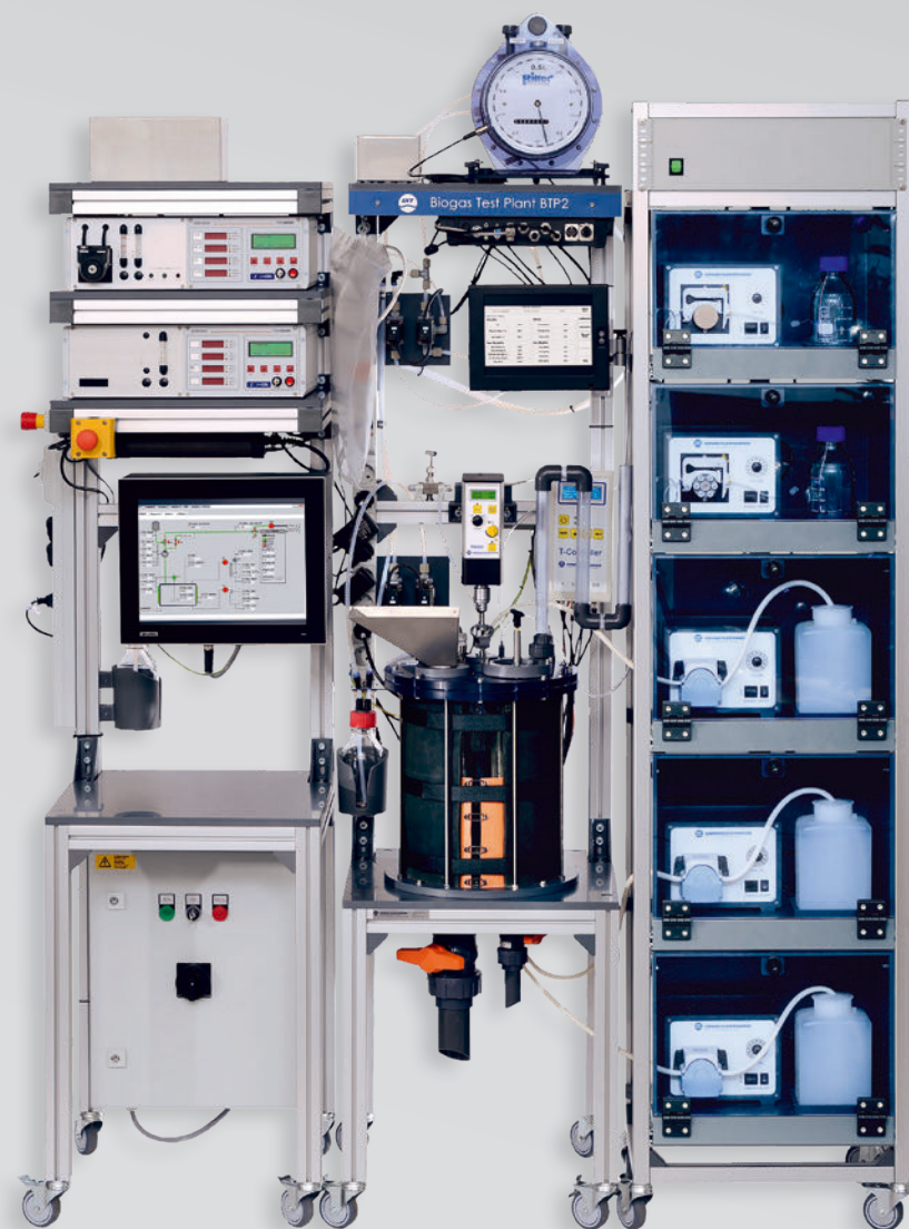
BTP2-control with pump modules
